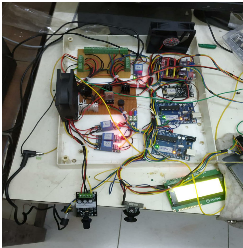
Fig 3.9 Fabricated circuit for both motion control and ECDM process
